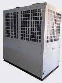
Air source heat pump is meant for swimming pool heating & cooling. It applies titanium heat exchanger & heat pump technology which can move heat from atmosphere to pool water. It is helpful to get better performance in low temperature. Heat pumps are easy to install & maintain. Standard capacity range available up to 200 kW; higher capacity available on specific request.
